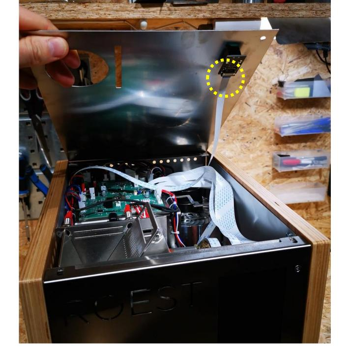
Loosen this bolt that connects the side panel to the roaster. Don't take it all out. Just loosen.
