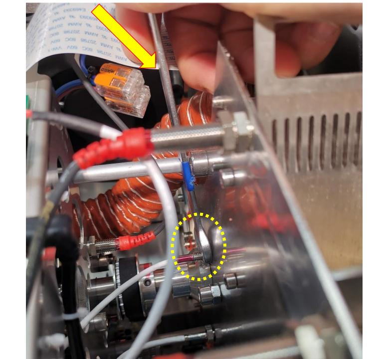
The new sensor has a nut that makes it possible to adjust it to the same length as the old sensor.
