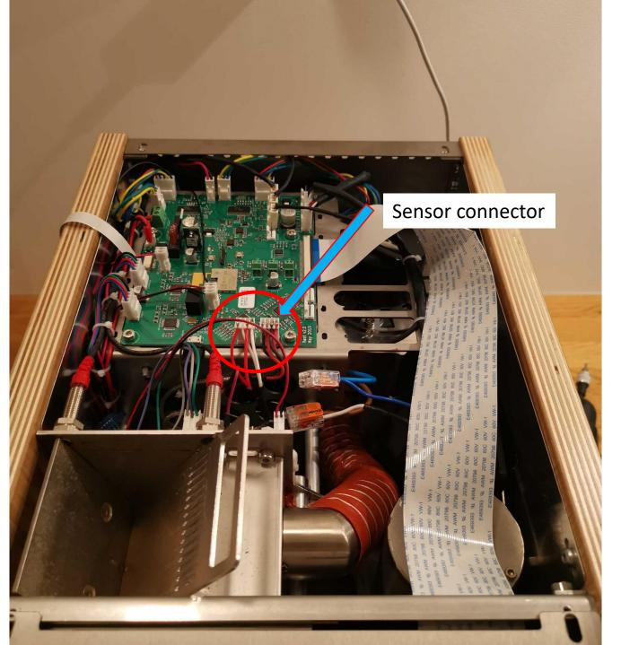
If they are soldered just check the connector. If they are not soldered you can press down the cables with a screwdriver. Like below.
